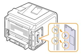
Push the DIMM straight into the DIMM slot until it snaps into place. Make sure the latches fit over the notches located on either side of the DIMM.
